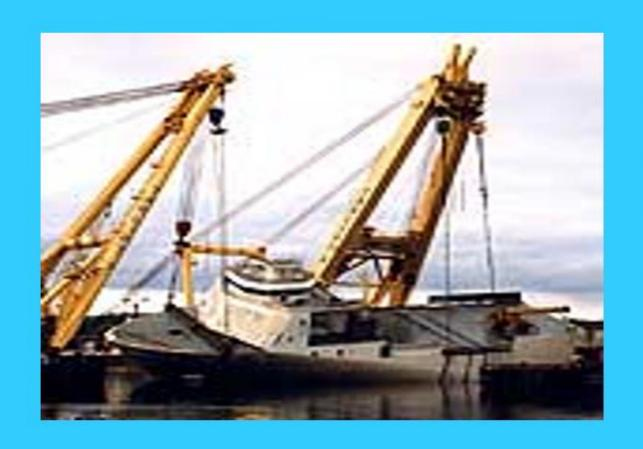
A salvage vessel has been equipped with heavy derricks to lift wrecks from the seabed.
