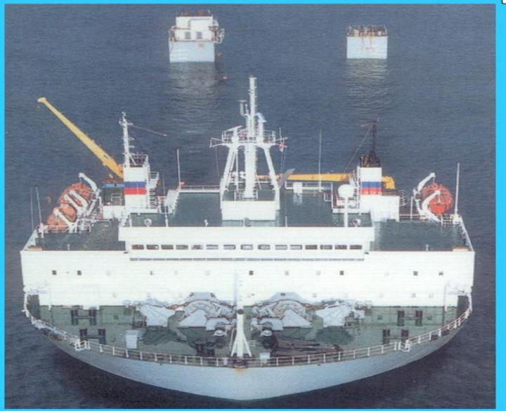
A semi-submersible heavy-load vessel is loaded by *submerging* it first.
